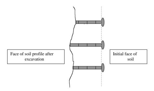
Fig. 2. Diagram of a section through the profile wall to illustrate the use of marking bolts to gauge the depth of excavation.
