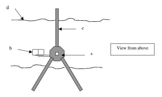
Fig. 3. Diagram of the camera jig. a) ratchet to hold vertical support for the camera; b) camera with viewing screen uppermost; c) supporting legs; d) profile wall of soil pit.
